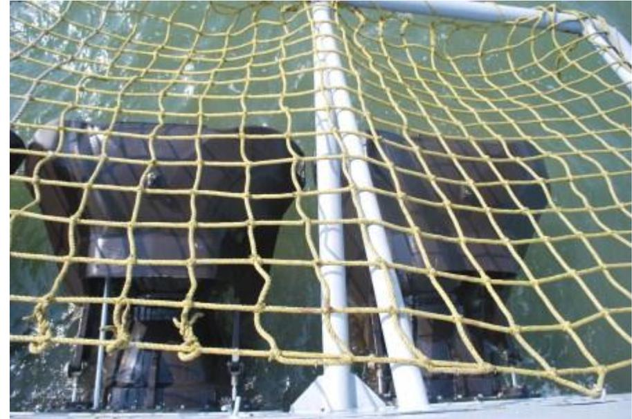
Two of the three HamiltonJet HM811 Water Jets of the INS Cankarso. The Cankarso is a Water Jet Fast Attack Craft (FAC). The propellers are actually fitted inside pipes through which water is pushed out at high speed. This also makes the Water Jet FAC much quieter. ([Stratpost](#))
