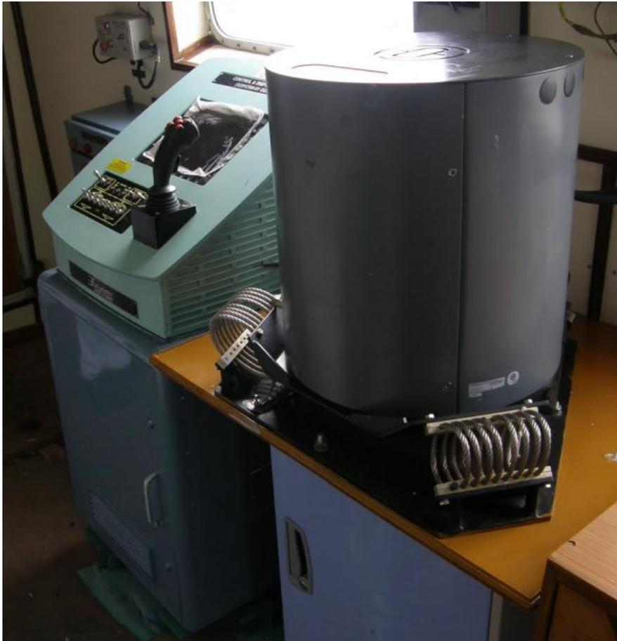
The gun controls for the CRN 91 cannon, and the spring-mounted gyro in the bridge ([Broadsword](#))
